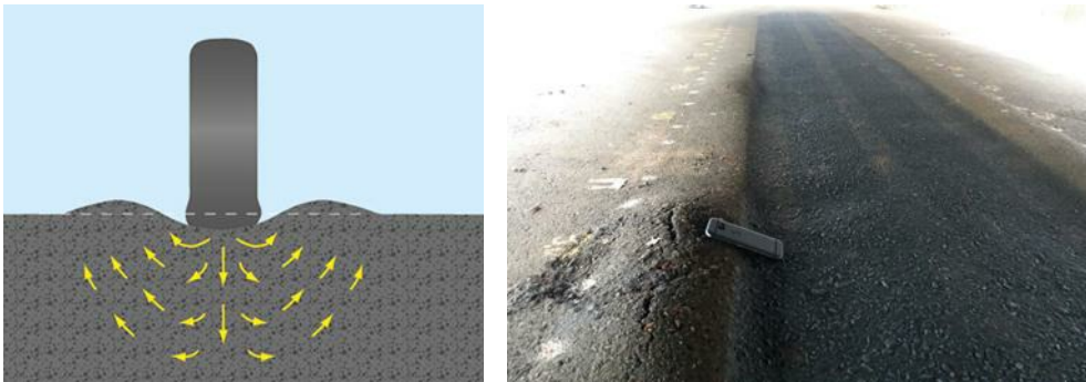
Figure 26 Rutting process caused by shift in tensions due to decrease of stiffness in the pavement materials.
